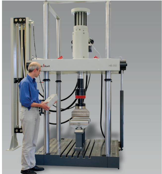
Fig. 2: Four-column HB250 for materials and components testing
