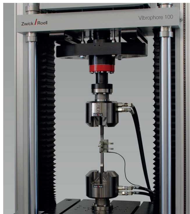
Fig. 2: Integration of makroXtens extensometer (top) and Clip-on extensometer (bottom) for static tensile tests
