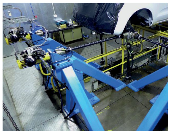
Fig. 2: Multi-axis test rig (Image: © Ford)
