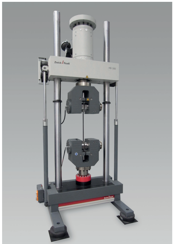
Fig. 2: High cycle fatigue tests on wire strands to ISO 15630-3
