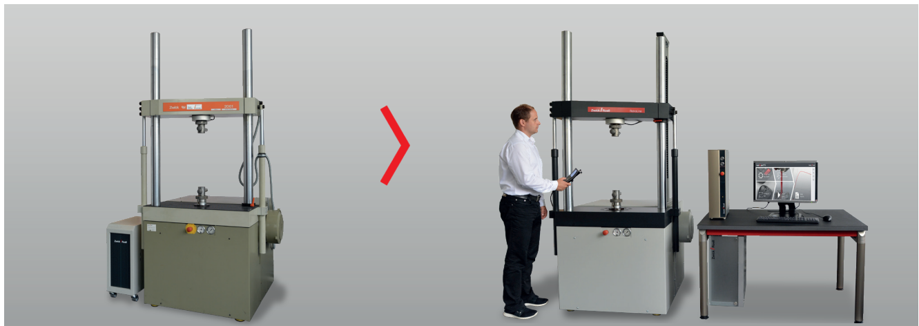
Fig. 1: Modernization of a servohydraulic testing machine with testControl II as well as testXpert Research testing software
