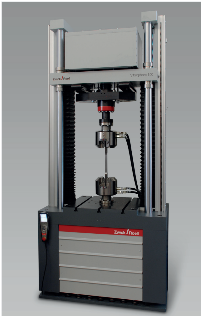
Fig. 1: Vibrophore 100 high-frequency pulsator with hydraulic wedge grips
