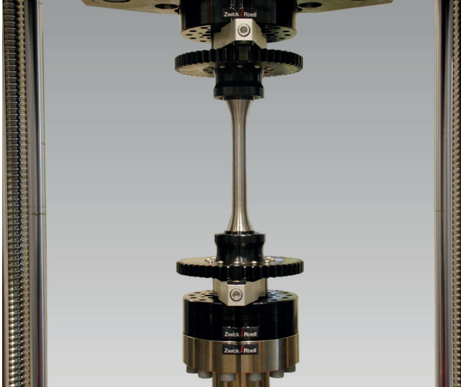
Fig. 2: Round specimens with quick-action clamping device
