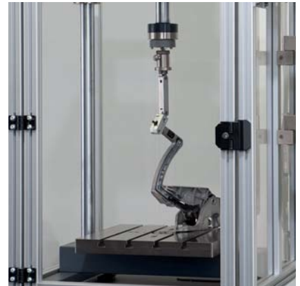
Fig. 4: Fatigue testing of an emergency brake lever
