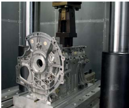
Fig. 1: Fatigue tests on the engine block
