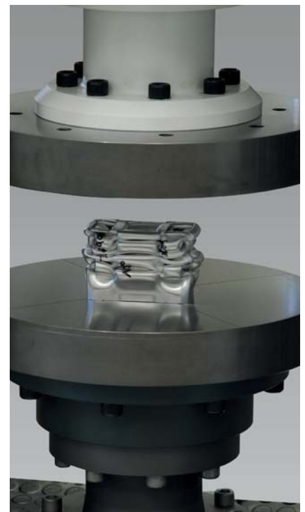
Fig. 1: AllroundLine materials testing machine with two test areas for tensile and compression tests on body components
