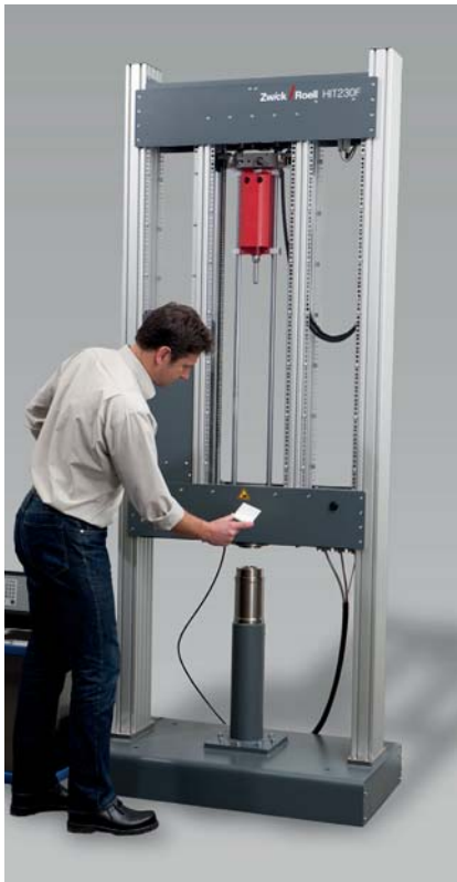
Fig. 2: HIT 230F drop weight tester
