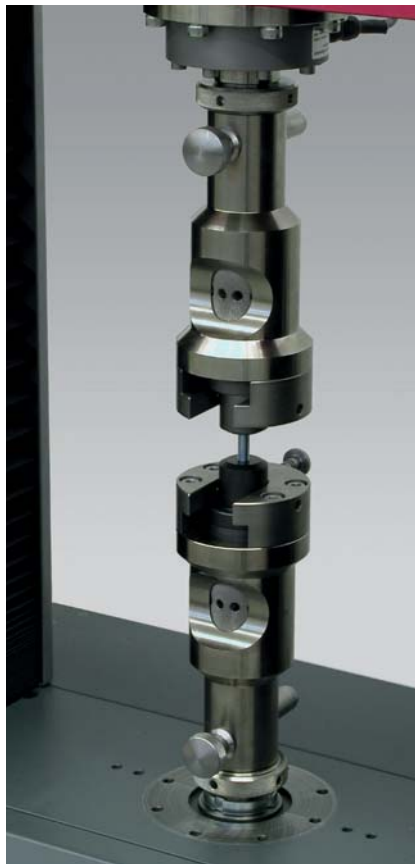
Fig. 1: Static tensile test on screws
