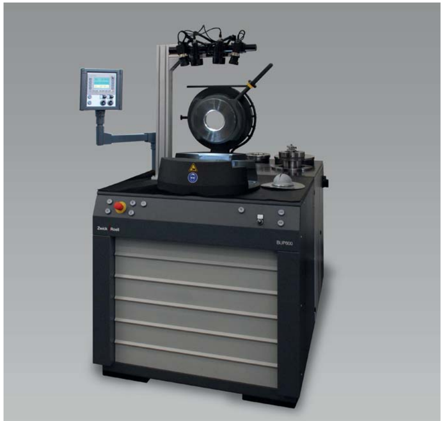
Fig. 1: BUP 600 sheet metal testing machine
