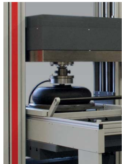
Fig. 2: Testing of pneumatic springs
