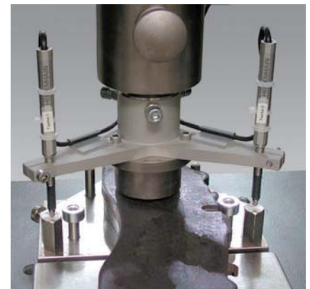
Fig. 5: Compression tests on brake pads
