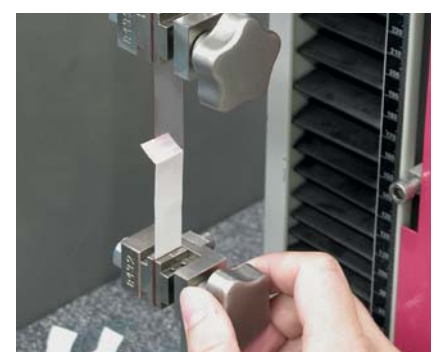
Fig. 7: Peel tests on adhesive strips
