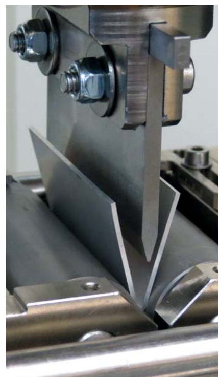
Fig. 3: Plate bending test to VDA 238-100
