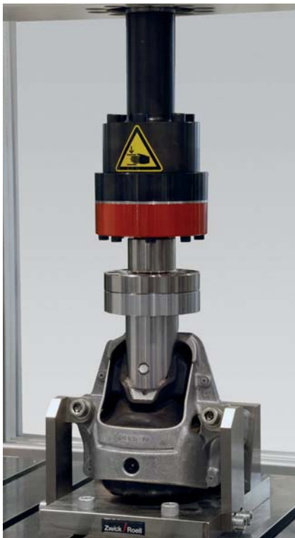
Fig. 1: Single-axis fatigue testing on engine mounts
