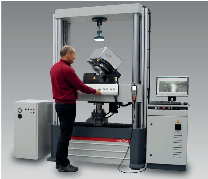
Fig. 1: Sheet metal testing machine with videoXtens
