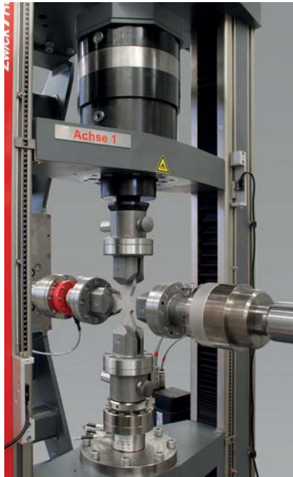
Fig. 2: Biaxial testing machine with superimposed torsion
