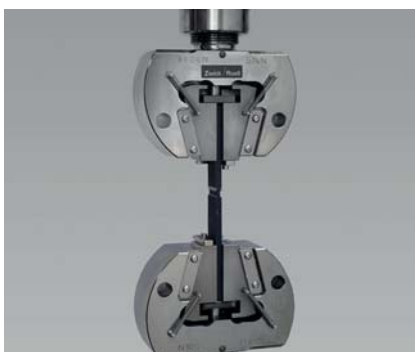
Fig. 2: Slotted specimen for adhesive bonding of two fiber composites in shear test
