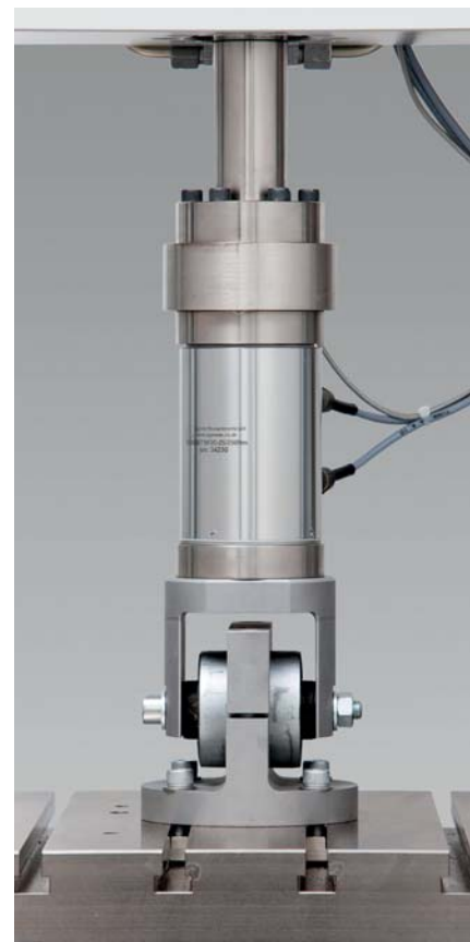
Fig. 3: Testing of rubber-metal dampers
