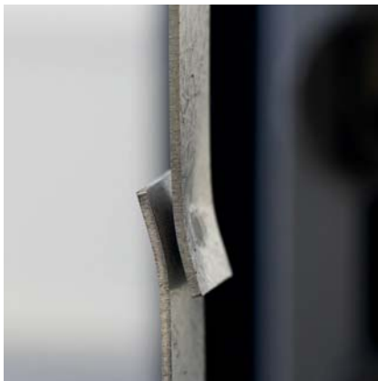
Fig. 1: Point welded specimen
