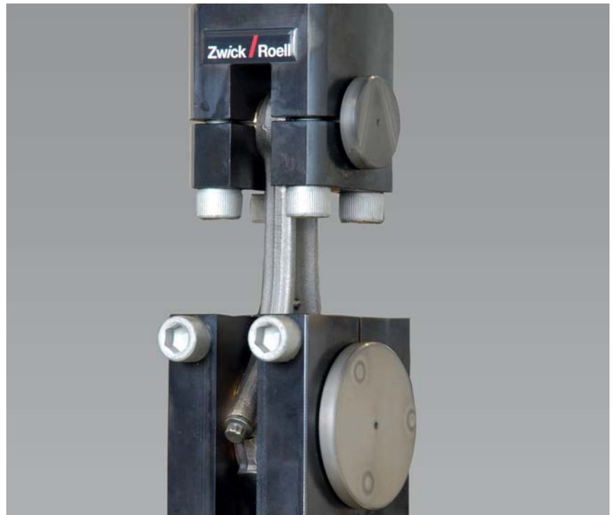
Fig. 1: Fatigue tests on connecting rods
