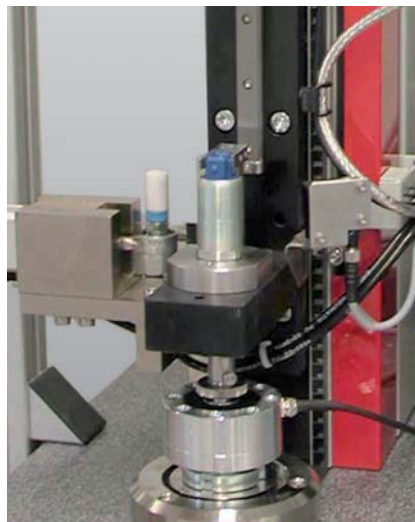
Fig. 1: Testing of electromagnetic actuators
