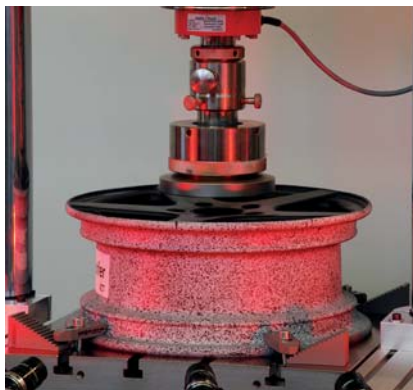
Fig. 4: Measuring full-surface deformations on a CFRP rim
