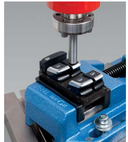
Fig. 2: Function tests on a window lifting switch element
