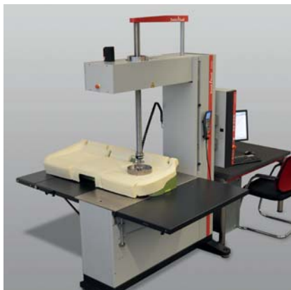
Fig. 1: Determination of indentation hardness of pre-formed flexible foams
