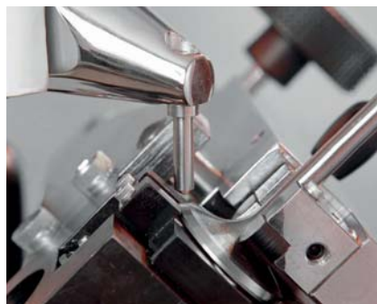
Fig. 5: Hardness testing on valves
