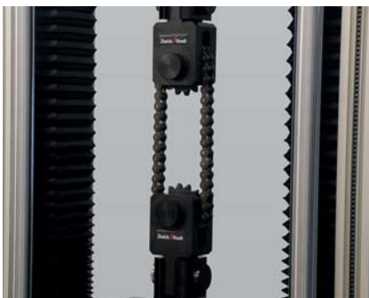
Fig. 2: Fatigue tests on engine chains
