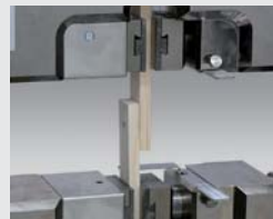
Tensile shear tests on wood joints
