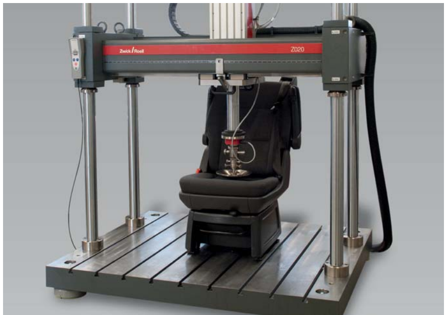
Fig. 2: Flexible test bench for characterizing seats
