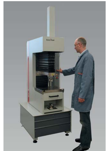
Fig. 5: Push out test for riveted joints
