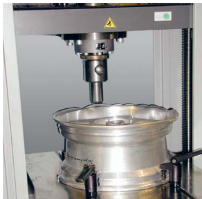
Fig. 3: Testing axial deformations of the rim flange
