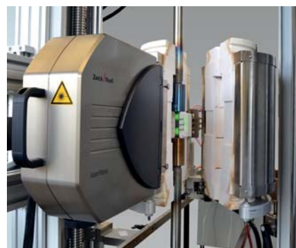
Fig. 4: High-temperature furnaces can also be retrofitted
