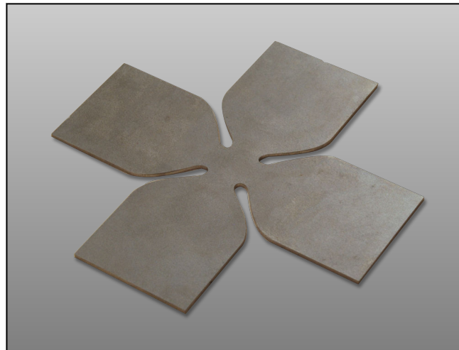
Customized cruciform specimen
